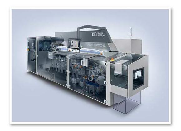
MKC - the continuous high-capacity cartoning machine
