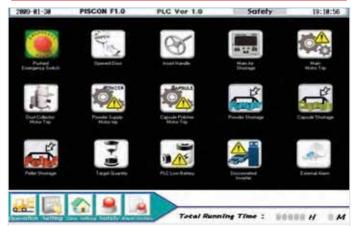
In the event of a machine stop by an alarm, it is easy to check the related alarm at a glance. The diagnostic display gives reason and solution for the activated alarm so the operator can quickly resolve the issue without engineer intervention.
