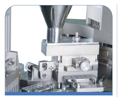
The Pellet device is for filling pellets into hard gelatine capsules. It is designed to minimize weight deviation so the supply of pellets can be easily adjusted to achieve the target weight.
