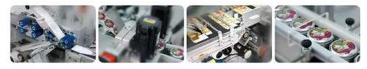
A732 Top & Bottom Labeling System is a system suitable for the top and bottom labeling on bottles, boxes, blisters, and other flat products, featured with high registration precision and easy adjustment operation.
