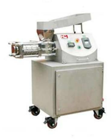
**Usage:** mix powder material, excipients and moist bonds to extrude compact cylindrical granules, which is prepared for spheroid zing pellets
