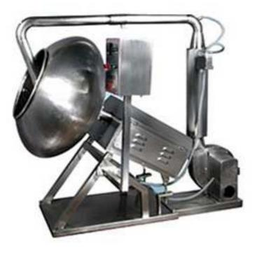
Coating pans offered by us are manufactured by us are used in the pharmaceutical industry for covering tablets and confectioneries. They are systematically designed after careful study of rotational speed, angle of inclination of pan volume and temperature.
