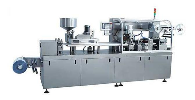
Roller-Plate type blister packing machine is a kind of blister aluminum (PTP) / plastic (PVC) compound sealing packaging equipment, It can pack the material like the drugs ( tablets, capsules ) food, medical equipment, health products, electronic components and so on, as using positive pressure forming, rolling sealing, it has a blister crisp, smooth forum features.
