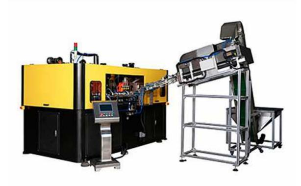
Automatic linear blow molding machines which are applicable in a wide range of PET packaging practice, such as for water, beverages, edible oil, food, pharmaceutical products and cosmetics, etc. With more than 10 years experience in developing and producing blow molding machine as well as the advanced technology absorbed domestic and abroad, we have developed with our constant innovation dozens of high speed and high precision equipments which have won the top reputation in the field.
