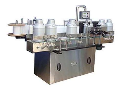
The Om Bhagwati Labelling Technologies's Automatic Vertical High Speed Sticker Labelling Machine Model SBSL-150-B, is one of the most user friendly. The Machine incorporates latest sophisticated Micro Processor Control Label Dispensing system with user friendly Sensing system for Label and Product. The Machine is suitable for Labelling on Round Bottle, Jars and other round objects. It is capable of Labelling up to 150 Products per minute depending on products diameter and label size.
