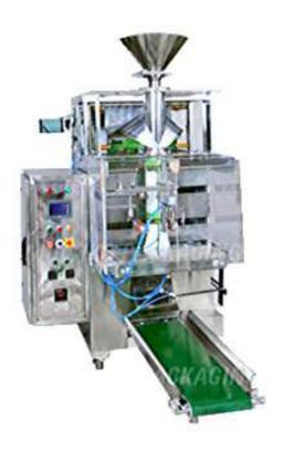
The MK-405 is a vertical form, fill and seal packaging machine designed to package various grains and snack products. This VFFS packaging machine is equipped with linear weigh scale and operates with electromagnetic clutch and it uses linear type weigh scale dosing system to produce center sealed pouches also commonly known as pillow pack or fin seal type pouches / bags.
