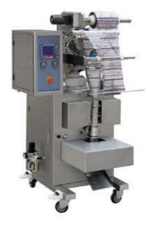
The machine is composed by feeding barrel, rotary measuring cup feeding equipment, thin film supply equipment, thin film molding machine vertical heat sealing equipment, horizontal heat sealing cutting equipment electric-control part, machine body part equipment ect. All the parts that contact with packing material is (304)stainless steel
