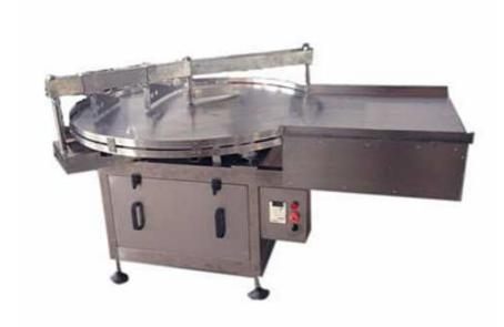
ZX-3 rotating bottle-feeding machine adopts frequency speed. Reduction gear drive work table rotating so that containers automatically enter into the conveyor road under the rotation force, together with the packaging production line. It saves labor and improves efficiency. This machine does rotary movement through frequency control so that empty bottles have access to conveyor. It is ideal replacement equipment for manual operation.
