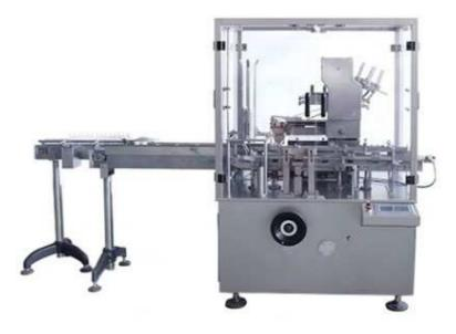
This machine is suitable for bottle (round, square bottle), into carton automatically. On line product feeding and detecting, carton opening and forming, products and leaflet push into carton, printing batch number, sealing carton with tuck-in or hot melt glue device. Automatically reject lacking of leaflet or product and finished product out.
