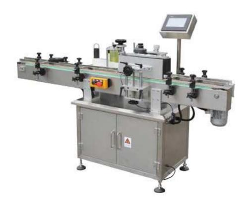
This Adhesive labeling machine used for food, medicine, cosmetics, electronics, hardware, auto parts, stationery, batteries, all kinds of oil round bottles, and a variety of different specifications of the packaging products, automatic labeling machine work.
