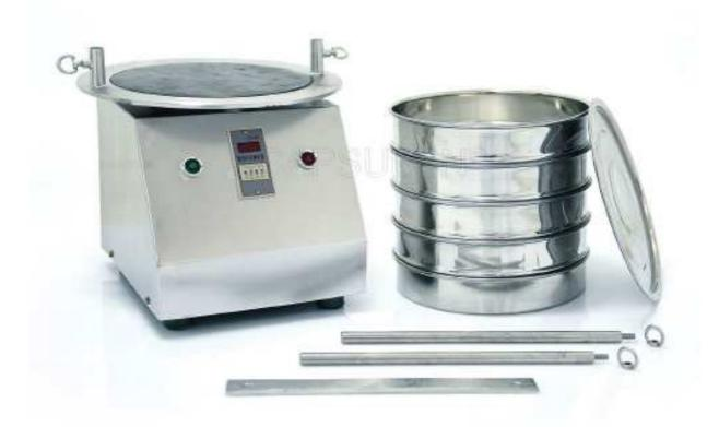
The machine is a small and light-weight laboratory separator capable of separating up to 5 classes (4 screens), it is widely used in pharmaceutical, food and chemical industries. It is the ideal equipment that is used to sift the materials such as granule, particle, slice, flake and powder. It works with no vibration of bottom machine body stand, low noise and energy consumption, no dust flying, high efficiency and it is convenient to carry, clean and maintain.
