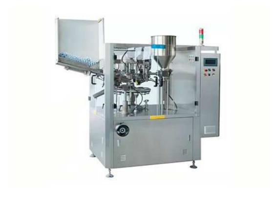
This machine is mainly used for filling and sealing soft tube which is widely used in the packaging of chemical industry and others
