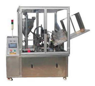
This tube filling and sealing machine is widely used in pharmaceutical, cosmetic, food and chemical industries etc. It is applicable in various aluminum plastic compound soft tube, plastic soft tube which fill pack all kind of Such as ointment, adhesives, AB glue, Neoprene, epoxy glue, skin cream, hair cream, boots oil, toothpaste and else liquid, lotions and cream etc.
