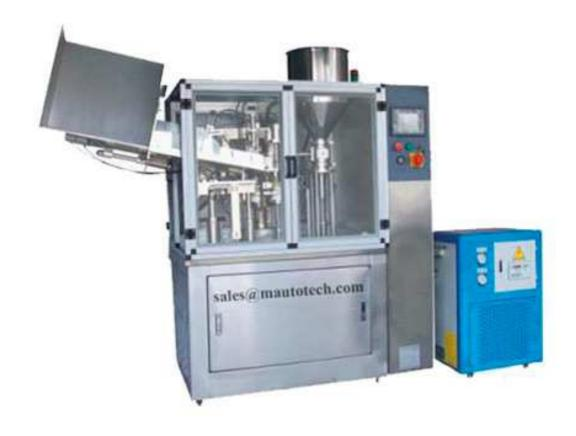
First manual or automatic insert tube into tube holder, the tube holders will rotate with the rotary table so that they will be positioned at different work stations.
