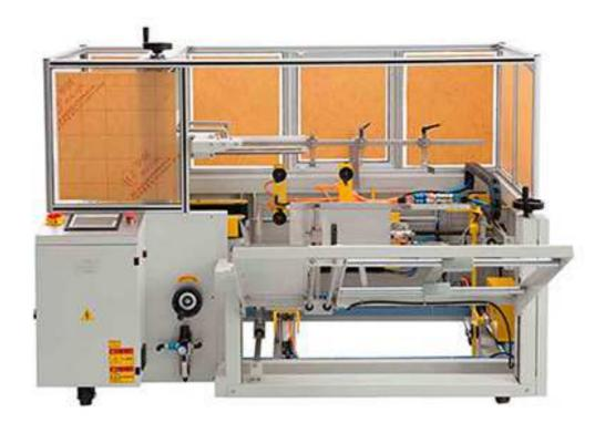
The automatic erector machine is used for the forming and sealing of cartons. The maximum opening speed of the vertical opening mode of the machine can reach 12 boxes per minute. It is usually used in conjunction with the sealing machine, packing machine and other equipment to form an automatic packaging production line.
