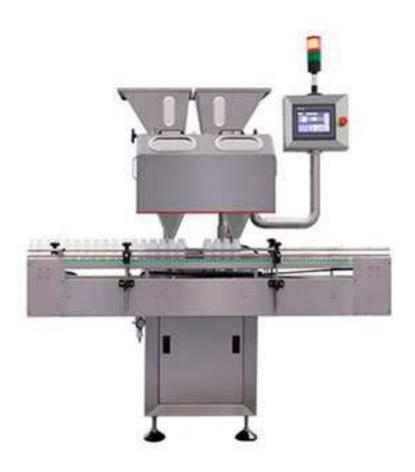
RQ-DSL-16 Automatic electronic counting machine is suitable 3-25 mm tablets, pills, #000-#5 capsules and etc. After feeding the material, using the device to close from the bottom to the top, can effectively avoid the damage to capsules or tablets. This 16 channel counting machine adopts tempered glass window, can check the machine's blanking process, if there is a fault, can adjust it in time.
