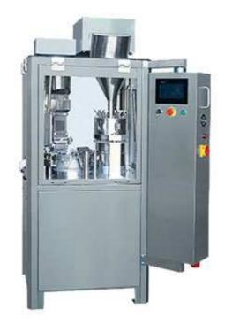
Type NJP-800 Auto Capsule Filling Machine is designed opposite to the normal models (With open style in dosing station and turret) in Chinese market, and it has been developed to fully enclose stations to ensure their flawless performance. And adopts the advanced technology at home and international similar products, The whole machine appeared as Humanity, Automation, Stability, Beautiful. And in accordance with to CE, ISO and GMP international standard.
