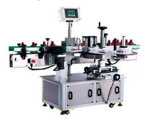
The one-sided automatic labeling machine is suitable for side labeling of square or flat bottle shaped objects.
