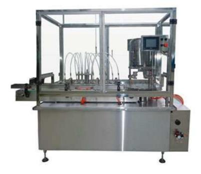
This monoblock vial filler capper is mainly used for filling and capping 10ml-100ml penicillin or glass vials.
