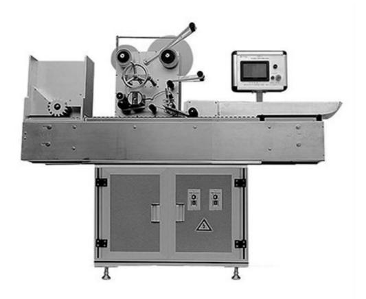
This blood tube labeling machine is used for medical disposable blood collection tube labeling process. The machine is composed of product transfer system, label machine, packaging machine, programmable logic control panel, electronic panel and other advanced functions, with accurate precision and robustness, to ensure the efficiency and effectiveness of the production process. All the safety parts of the blood tube labeling machine have been taken into account, including all the moving parts.
