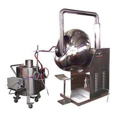
This machine is used to carry out sugarcoating and film coating to the core of Chinese traditional and Western medicine tablets. It integrates strong power, weak power, hydraulic and pneumatic. It is new type equipment improved on the basic of original common type sugarcoating machine.
