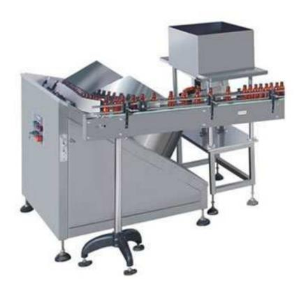
This machine is suitable to unscramble general round and flat plastic bottle, such as eye drop bottle, syrup bottle etc. And other bottle type can be customized in this machine system. It is able to unscramble disorder bottle to stand right side onto the conveyor. All contact parts is made of SS304, accordance with GMP regulation.
