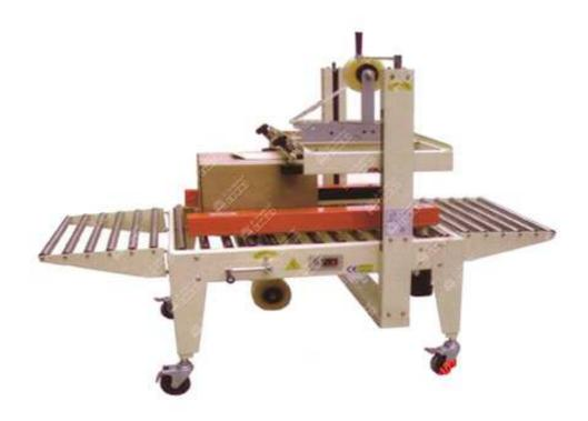
Semi-automatic carton sealing machine adopts the adhesive tape sealing carton sealing, which is economical and quick to adjust. It can complete the upper and lower sealing actions at one time, and can also use printing tape to improve the product image.
