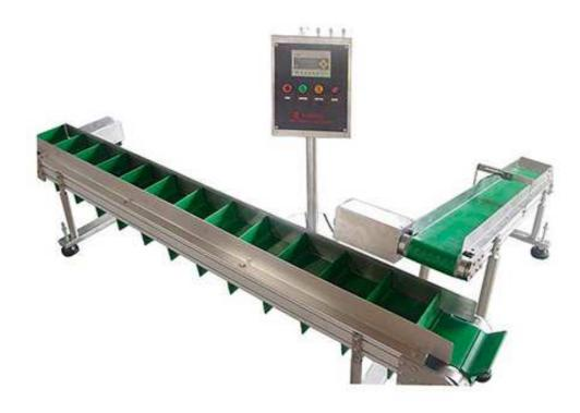
Be suited for various bag counting, adjustable setting of running speed and counting numbers, and no limit convey amount. Convey function can be adjust by PLC system.
