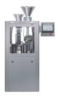
NJP-200C Automatic Capsule Filling Machine adopts butterfly valve-type powder feeding, and is very suitable for drug powder with poor liquidity, including Chinese herbal medicine and Chinese patent drug, due to that its vibration unit equipped will force the powder to run down, which has solved problem of failing to feed in powder that often happens in the traditional screw feeding device because of the poor liquidity of powder.
