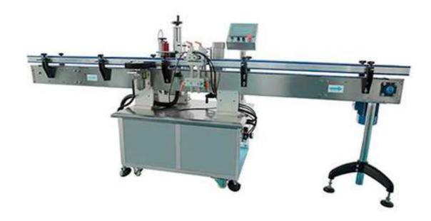
This machine is suitable for round bottle half wrap or whole wrap, artificial bottle to take bottle, also can connect machine use, paste one label or two labels at a time, apply to a variety of material circular labeling.
