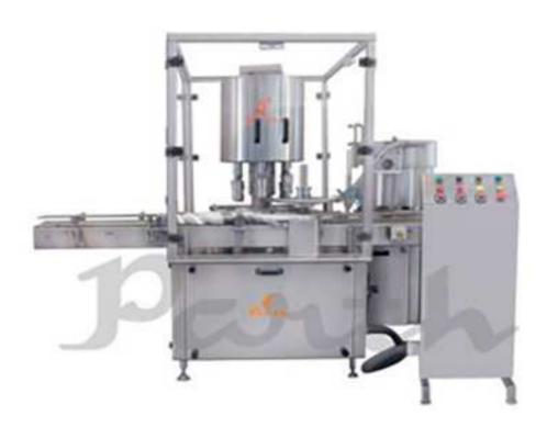
The Automatic Screw Cap Sealing Machine is precision built on sturdy welded MS frame completely enclosed in stainless steel sheet and doors are providing to facilitate the servicing of machine.
