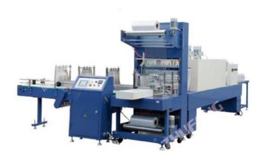
The machine is automatic mantle heat-shrink packing machine is widely used in square, round, flat shape bottle plastic film shrink packing for beverage, food, medicine, chemical industry, without bottom bracket, without carton boxes, packing perfectly, low cost, do not take place, easy to transport.
