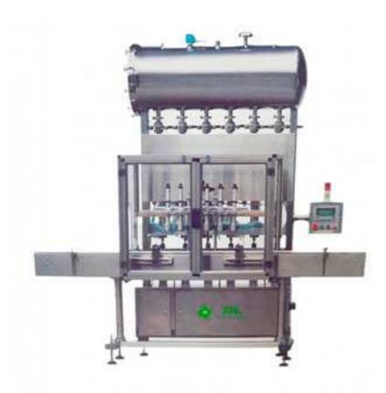
AV6T-6G is improved and developed from the same product overseas, combining new design and advanced technology, and multiply parts of function. Make the product more convenient in operate, adjustable, clean and maintain. The volumetric pump is high filling precision and stability. It is widely applied to daily chemical and oil product, filling more kinds of light and heavy liquid. Adopt the pneumatic cylinder driving, easy to adjust the filling volume, compact and good appearance.
