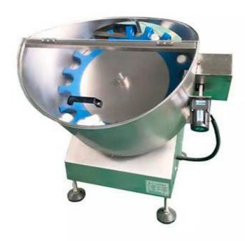
The motor drives the sorting flower plate. The bottles in the container begin to rotate from the under part to the upper part of the bottle sorting plate by the semicircle groove of plate and the guiding rod. The bottles in the semicircle groove are picked up continuously by the plastic turning strips, which are fixed on the bottle exit, turning around constantly. Then all the bottles, with mouth up, move in order along the conveying belt to the filling station.
