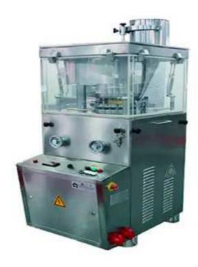
This machine is a continuous automatic tablet press for pressing granular raw materials into tablets. Rotary tablet pressing machine is mainly used in pharmaceutical industry and also in the chemical, food, electronic, plastic and metallurgical industries.
