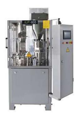
NJP800 Automatic Capsule Filling Machine can be widely applied to the powder, grain, tablet and pellet filling. The control panel of the machine is supplied with touch screen control (PLC) control system. All powder contact parts are in S.S. 316 qualities.
