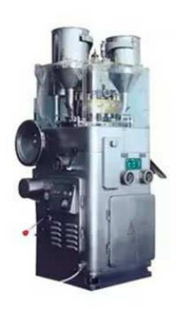
ZPW21 Rotary tablet press is designed for pressing tablets from various kinds of granular materials. ZPW21 Rotary tablet press can press not only round tablets but also irregularly shaped tablets, double-layers and annular tablets. The tablets may have the impressed letters on both sides. The turret carries 21 sets of movable-punches and dies. So, 21 tablets press will be pressed for each rotation of the turret.
