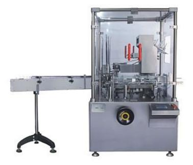
Developed on the basis of advanced technology at home and aboard, vertical cartoning machine is a high-tech product integrating mechanics, electronics, light and gas. Vertical cartoner is applicable to automatic feeding and cartoning of various blister-formed or bottled items.
