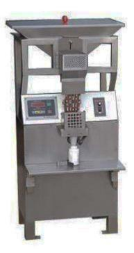
It is a professional hard capsule counting machine, which also equipped automatic counting machine. It has features of operation and the counting speed can be adjusted by manual loading the bottle speed. The bottle will stop counting when the one bottle is full and it can start counting when empty bottle is loaded.
