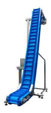
The PU belt conveyor is well suitable for the free-flowing products in the food, agriculture, cosmetic and chemical industry.
