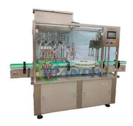
This series filling machine are suitable for filling cream, ointment, lotion, shower, gel, and liquid products etc. The machine can be used for traditional cylinder filling power, also can adopt servo motor as power filling, Compared with the traditional cylinder, servo motor filling accuracy is higher, the accuracy can reach<±0.5%, it has the characteristics of high efficiency, high precision, high hygiene standards.
