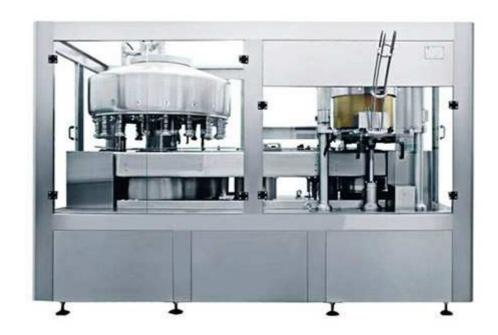
The machine is for vacuum filling and sealing of no carbonated drinks like juice/tea/coffee so on no beverage which is packed by pull-tab tin cans. It adopts mechanism, electric and pneumatic control technique, having the characteristics of automatic can-feed, automatic aluminum top falling, and no filling and sealing.
