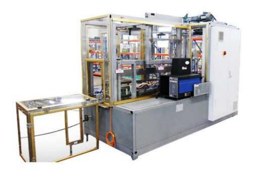
Hot-melt glue carton erector has been widely used to folding and forming cartons in different speculations before they are used in the beer, beverage and food production line. The capacity is 30-40 cartons per minute.
