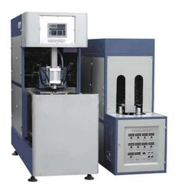
JN series blowing machine special program controller is a new generation multifunctional intelligent time relay specially developed fro bottle blowing machine customers by the company. Adopting 8 single chip machine data processing technology, it is programmed according to the working features of the bottle blowing machines. With the advantages of simple and convenient operation and reliable performance, it is the renewal products of digital reading time relay JS-14S and HD-48S.
