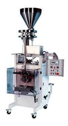
The ROTOR SERIES volumetric cup-fillers are the economical way to feed most of the granular and powdered products of all natures.
