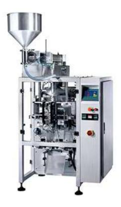
This is the description of automated filling equipment automatic filling machine for liquid JT-420L 10g/ 50g/ 100g/ 500g/ 1000g bag 10-70 bags/ min oil/ shampoo/ sauce/ jam/ milk/ liquid packing machine
