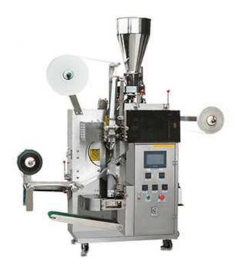
Automatic Tea Bag Packing Machine KS-T80 is the latest heat-sealing and multi-functional packing machine, which is featured at one-time packing of the inner and outer bag, and effetely avoiding hands in direct contact with stuff materials, and its high efficiency in packing 1800 to 3600 bags per hour.
