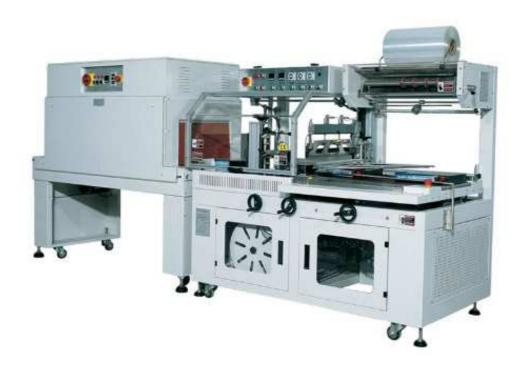
This automatic L type sealing and cutting shrink wrapping machine, widely used in assembly line work for large quantity package with high work efficiency, equipped with a pinning hole device, adjustable film feeding system and adjustable conveying platform, meets different requirements for different products and it has a kissing device for packing the small products.
