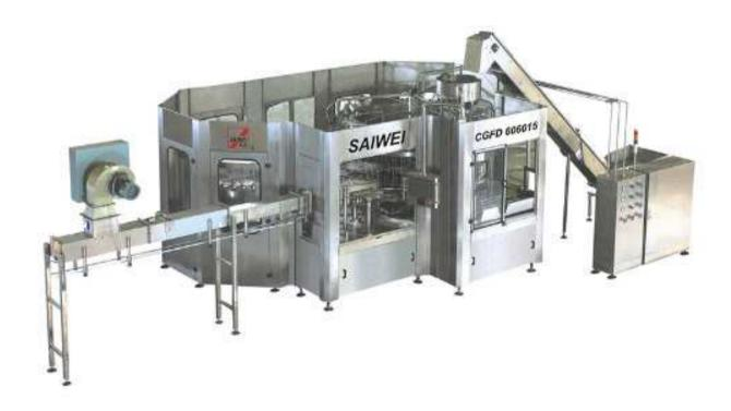
This kind of complete set of machine combines washing, filling and rotary capping functions in one unit, is a fully automatic and high efficiency liquid packing equipment.
