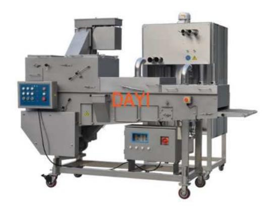
This Patty predusting machine can convey the products by the net belt, while the flour on the belt coated its bottom and the upper dusting flour coated on the surface. It can connect with Battering machine and Breading machine to form a different product process lines.
