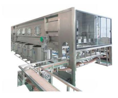
It integrates bottle washing, filling and capping into one unit. In order to achieve the purpose of washing and sterilizing. The washing machine use multi-washing liquid spray and-thimerosal spray. This thimerosal can be used circularly. The capping machine can cap barrel automatically.
